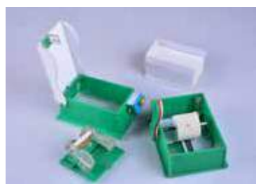
Token Dispenser which dispenses tokens with just one touch. It dispenses token when the user turns the handle on the side. This device is operated by pressing the button manually. The entire product is created using only recycled materials.
